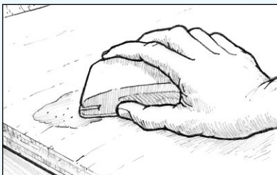
Figure 23 Sand cured fairing compound to desired contour.
